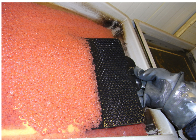
Eggs counter from organic fish production. Photo: ICROFS project RobustFish
